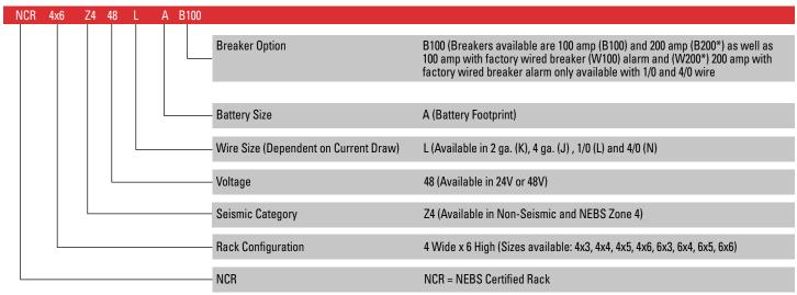
NEBS™ Certified Rack, 4 Wide x 6 High, NEBS Seismic Zone 4, 48V, for SBS 190F footprint with 100 Amp Breaker
